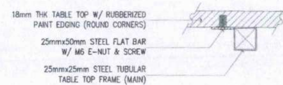
3 FRAME/FLAT BAR-BOARD CONNECTION DETAILS 2 SCALE 1 : 50 M
